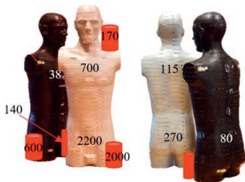
FIG. 4. Front and back view of setup 1 with reference dose rates (mGy). In the actual exercise the phantom closest to the source was an adult female ATOM phantom.
